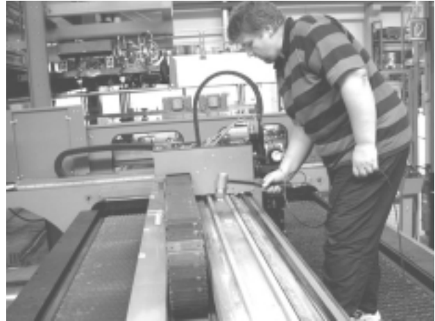
Figure 2: Impulse excitation of machine
